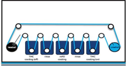
GE's proposed modular R2R pilot line for fabricating solution phase molecular layer-bylayer synthesis (mLbLS) reverse osmosis (RO) membranes. *Photo courtesy of GE Global Research*
